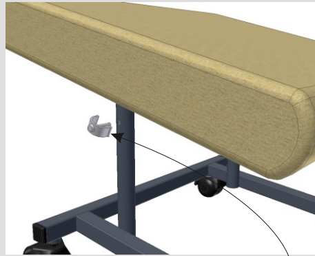
Height adjustable legrest with tube-locks to adjust height.
