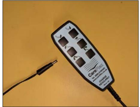
Fit the charging plug from the charger into the socket on the side of the handset.
