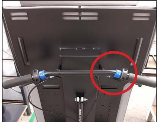
The lever on the right side of the push handle operates the Tilt-in-Space (TiS).
