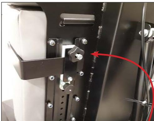
Turn the hand wheel to adjust lateral width, tighten the hand wheel to hold the setting.
